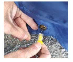
Place the seal behind the pallet tab and insert it into the two holes on the pallet cover. Then tighten very tight.
